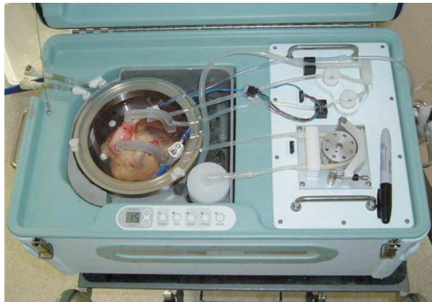
Fig 1. Heart Transporter™, a portable perfusion pump equipped with temperature and perfusion pressure controls, as well as a bubble oxygenator. After baseline analysis in situ, hearts were preserved in cold storage or with continuous perfusion using this apparatus. After preservation, hearts were reperfused with blood at 37°C using an isolated nonworking heart preparation (Langendorff) to simulate heart transplantation.
